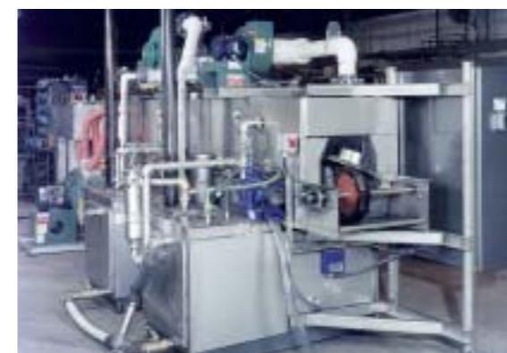
Rotor Rooftop Washer orients parts on angle and provides continuous part rotation for optimal cleaning and drying.
