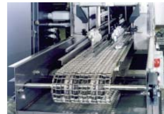
Brake Caliper Washer with guide rails to orient parts for optimal cleaning and drying.
