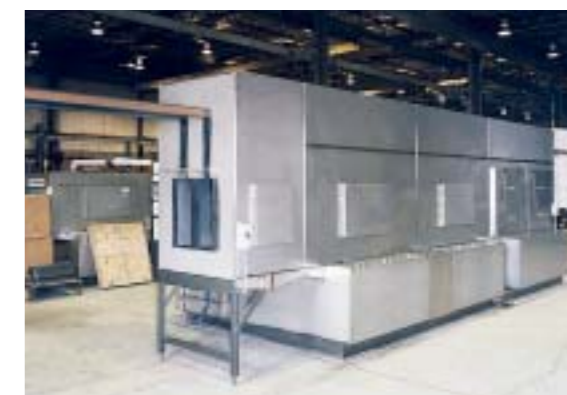
Overhead Monorail Washer Dual Track handles heavy parts.
