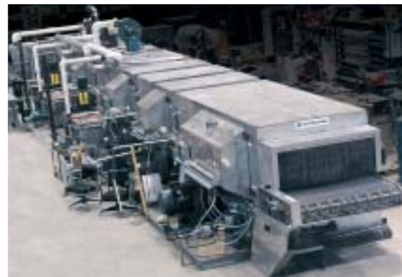
Wide-body Belt Washer for larger parts, sheet metal cleaning or high production multi-lane applications (machine shown has a 64" wide belt).
