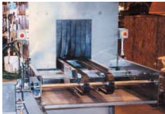
Dual-Strand Conveyor Washer accepts parts fixtured on pallets, in baskets, or stand-alone, for easy transfer and cleaning.
