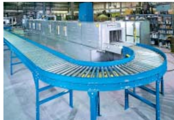
Multi-Stage Washer with Return Conveyor for the tough cleaning jobs such as buffing compounds. Return conveyor for automation.
